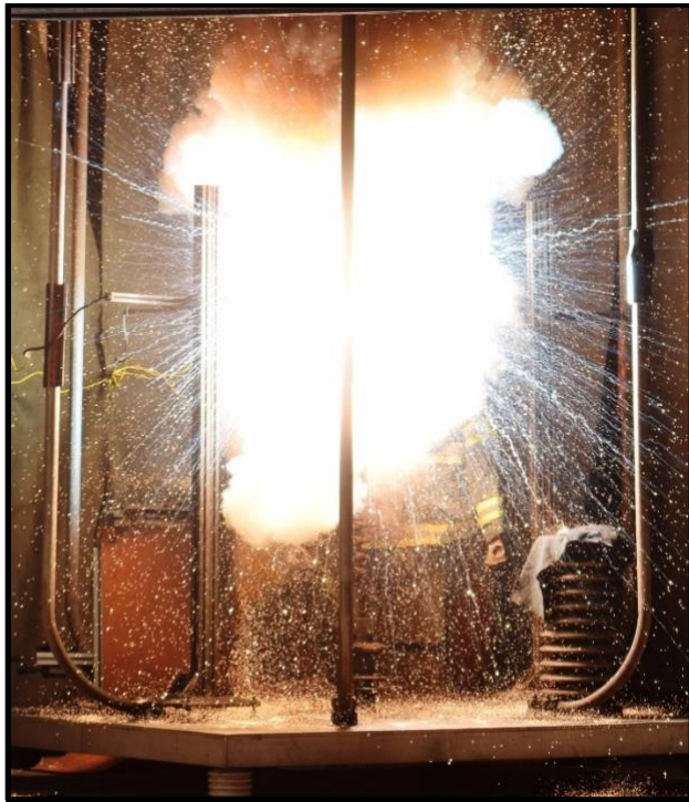
Figure 2: Simulated arc flash. PPE is subjected to 80KA for 70cycles/1.3seconds
