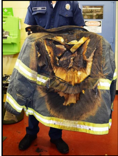
Figure 3: Effect of Arc Flash on PPE. The front of this coat is unaffected.
