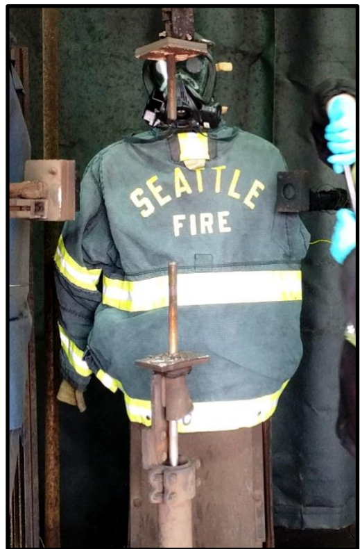
Figure 1: SFD Structural PPE with Facepiece, Flash Hood and Helmet. Metal rods in the foreground create the electrical arc flash.
