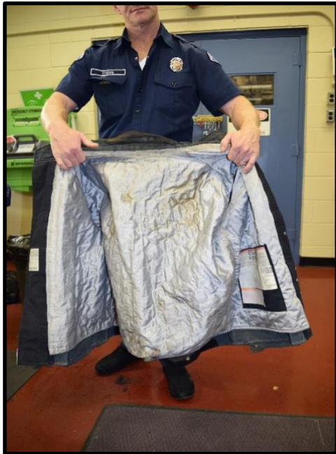
Figure 4: Same coat as in figure 1&3. This would be considered successful arc flash protection
